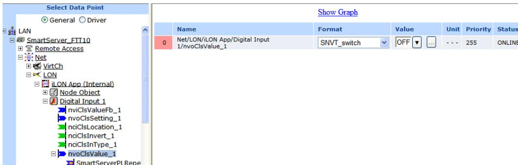
4. In the remote SmartServer tree (the tree for the SmartServer attached to the power line repeating network) on the same SmartServer, click the target data points that are bound to the source data point you selected in step 3. Observe that an **IP address** property appears on the Web page. This enables you to distinguish on which SmartServer a data point is located.
